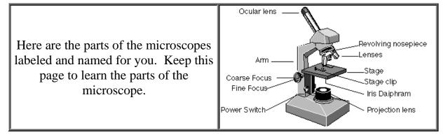
Adjustment mechanisms (Course Focus/Fine Focus) - an apparatus that moves the optic tube up and down to focus on the specimen
